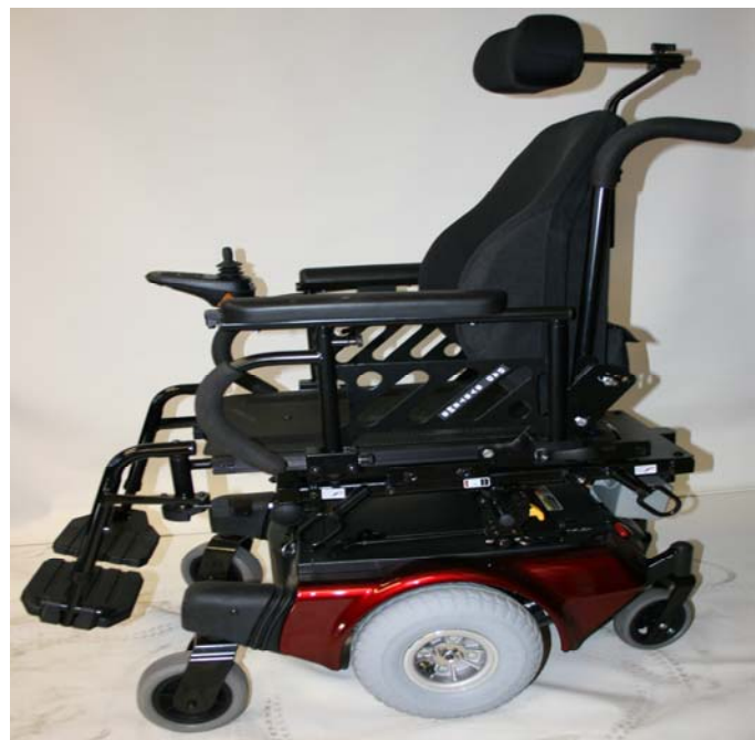
Shoprider 424M/Tilt with PSS-S-Seat Using Platinum Seat Assemble with Swingaway Footrests Mount on 424M with a Shoprider Tilt
