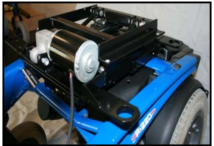
TILT INSTALLED ON TO THE BASE
