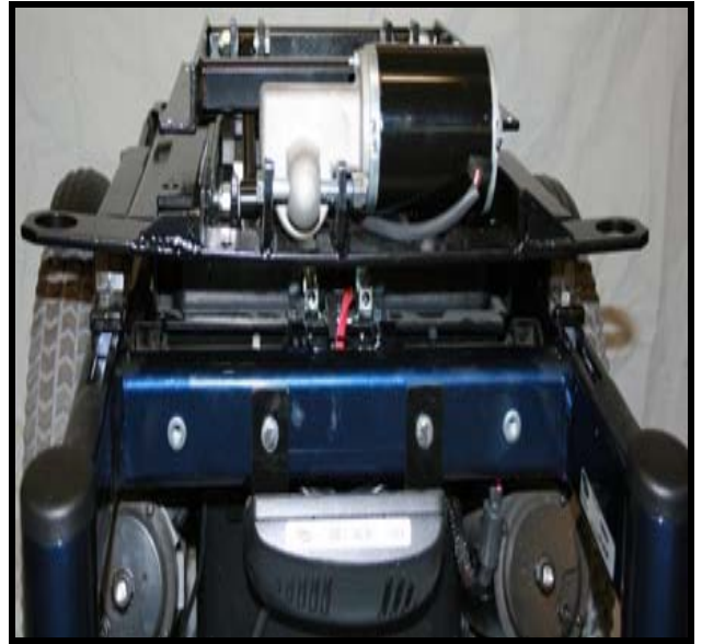
TILT INSTALLED ON TO BASE
