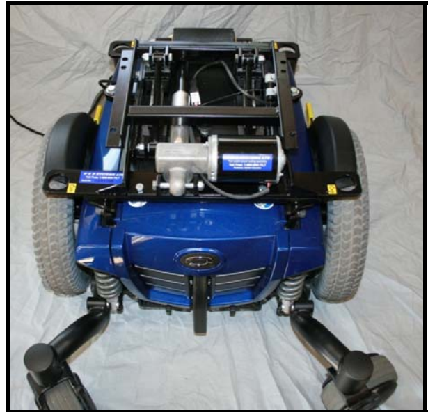
TILT INSTALLED ON BASE
