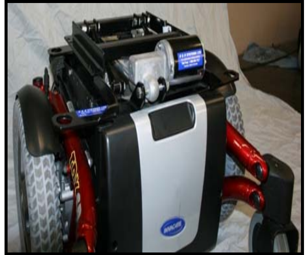
TILT INSTALLED ON TO BASE
