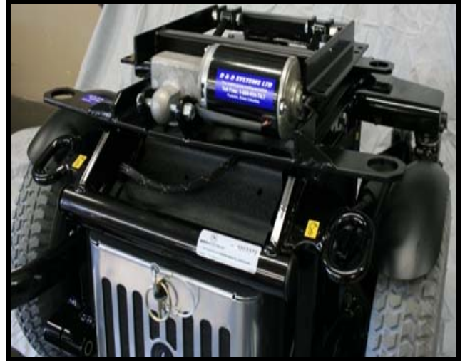
TILT INSTALLED ON BASE
